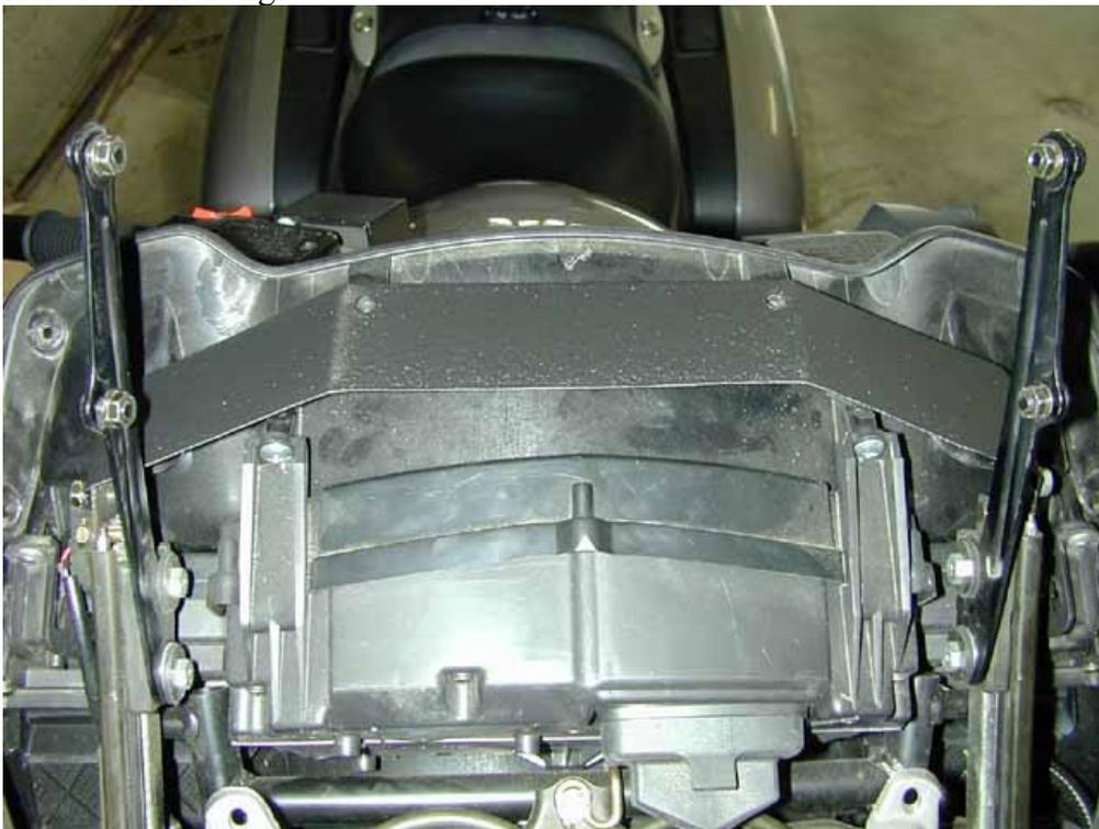
8. As you tighten the side bolts, align the support bracket holes with the channel clip holes. You may need to pinch the bracket back towards the plastic dash face as shown below.
