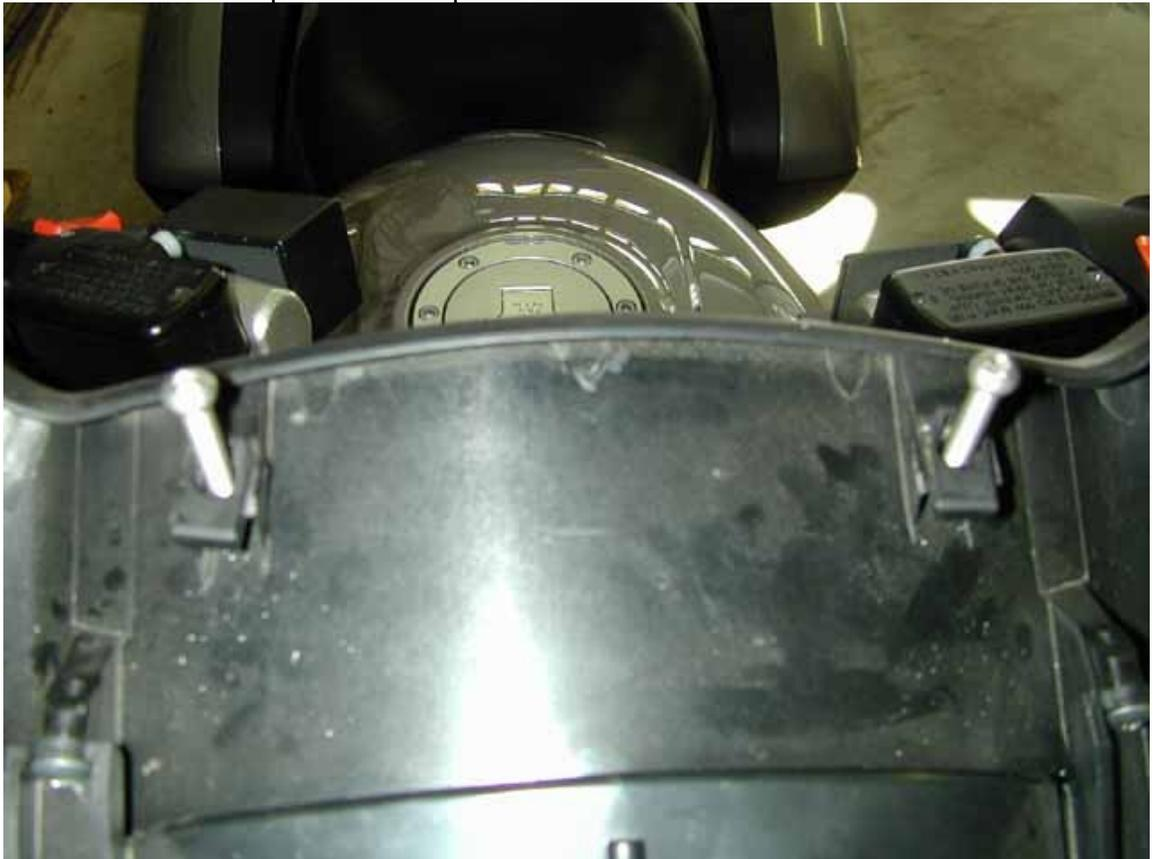
7. Now take the internal support bracket and align the two holes on each end with the holes at the top of the windshield's railing. You will have to remove one bolt but will reuse it when you mount the support bracket. While you are aligning and installing this bracket, be sure to check the alignment of the two holes in the
