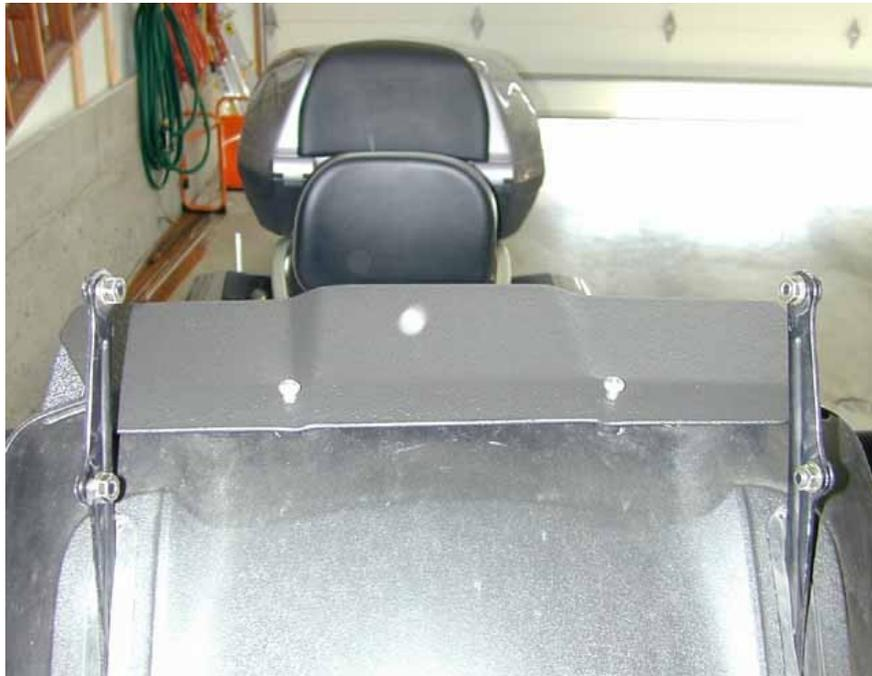
14. Now thread the replacement Phillips head screws into the dash strut holes and into the dash face plate until they're tight.
