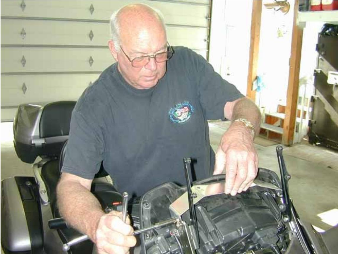
9. Replace the plastic dash cover on top of the dash and over the internal support bracket. Align the holes in the plastic dash cover with the holes in the channel clips below and the holes in the support bracket. You may again need to press the plastic dash face up towards the dash cover and the cover toward the face.
