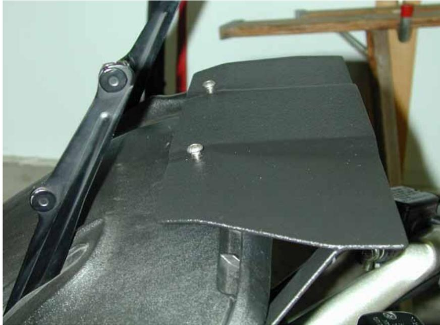
13. Tighten with an Allen wrench but do NOT over-tighten.
